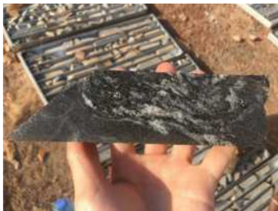
Zone of deformation and sulphide mineralisation
