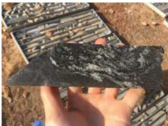
Zone of deformation and sulphide mineralisation
