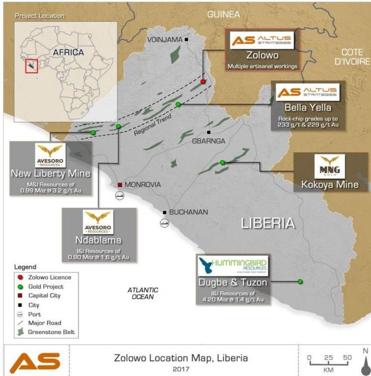
**Figure 2: The geology and location of artisanal workings of the Zolowo licence**
